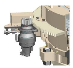
Hydraulic motor for setting adjustment and for opening the crusher for service and liner change
