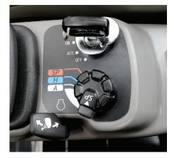
Operators can store up to 10 auxiliary hydraulic flow settings (and pressures as optional) to easily switch among different attachments with no need of any mechanical adjustment.
