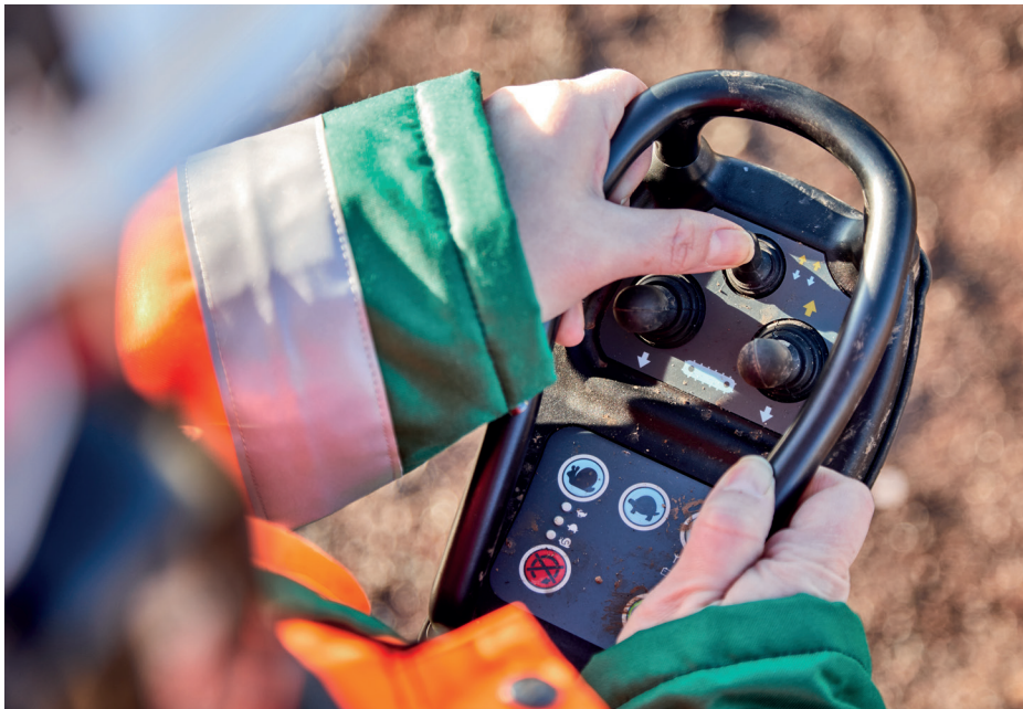
Remote controller for crawler tracks as standard.
