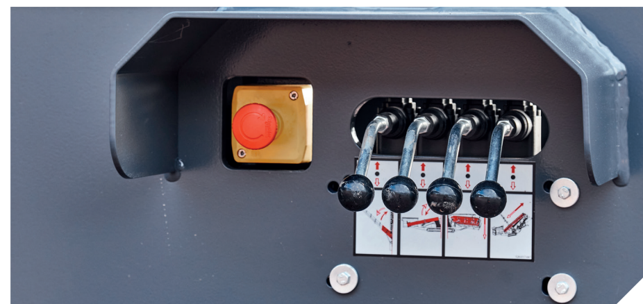
Six emergency stops, start siren, engine shutdown system and nip point guards for safety
