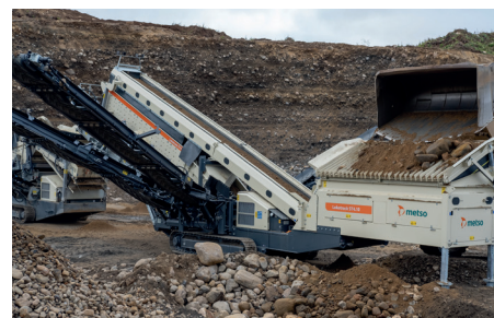
Large feed box allows closed circuit process.
