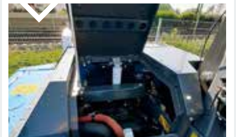
LOG-OUT TAG-OUT BATTERY MASTER SWITCH
