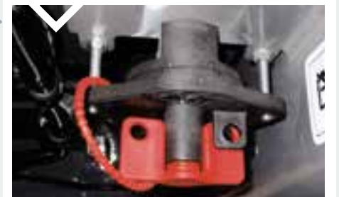
LOG-OUT TAG-OUT BATTERY MASTER SWITCH
