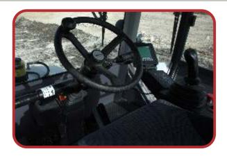
The operator station has an adjustable swivel seat with variable suspension for comfortable driving and excellent visibility in all directions.
