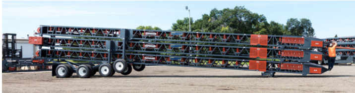
3 TRANSFER CONVEYORS IN A SINGLE LOAD
