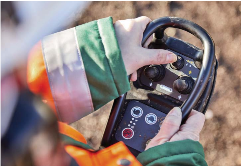
Remote controller for crawler tracks as standard.
