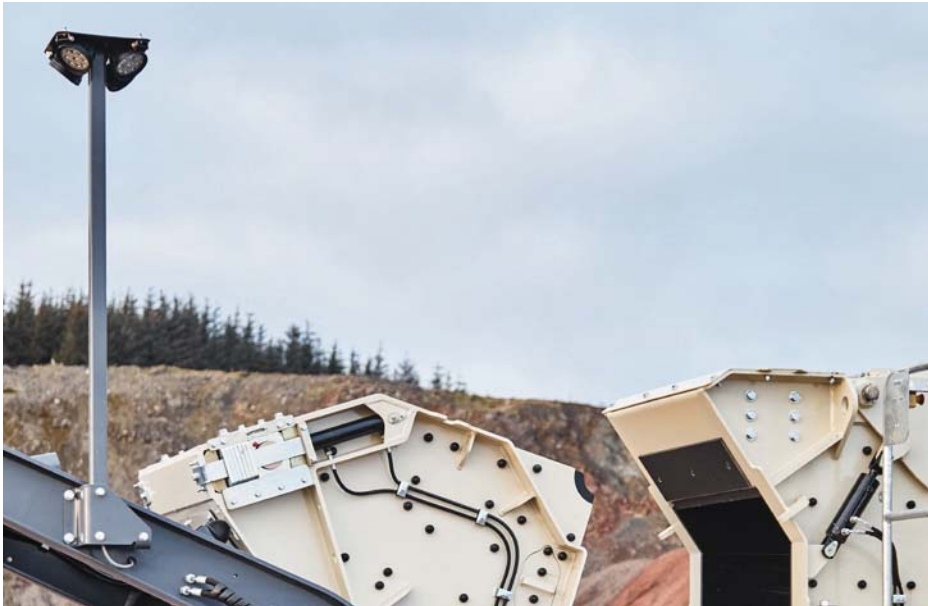
Working lights as standard for better work ergonomics and safety.
