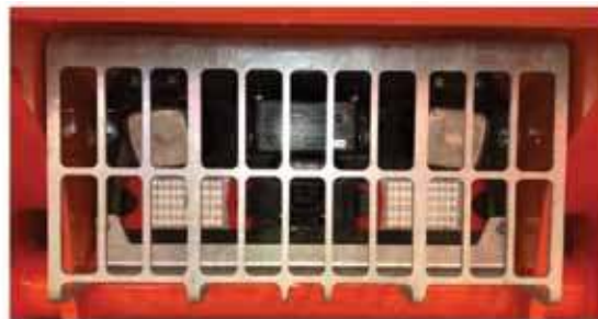
Rear plate with white noise alarm, LED revers light package, and light protection. Work light also available as halogen.
