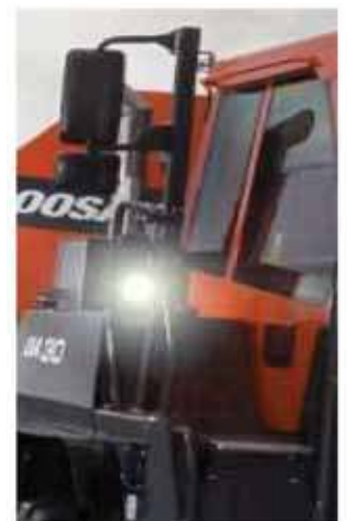
Rear and front work light on mirror arms, LED or halogen.
