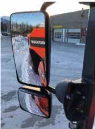
Headed and electrical adjustable mirrors.
